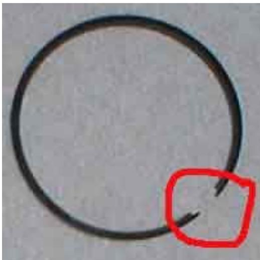
Next you have to locate the ring end gaps correctly on the piston. Look closely in the piston ring grooves, you will see a small pin in the groove, the ring ends go right at those pins. If you have 2 rings the pins are NOT in the same location for both.
